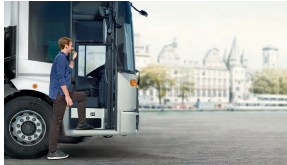
Two steps for improved ergonomics: the low-entry design of the Econic makes getting in easier and getting out safer.
