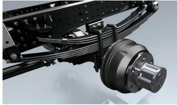
The braking system provides firm intervention on the road and maximum deceleration in more demanding situations. Well protected against dust and dirt, the system features front and rear drums, ABS and electronic brake force distribution (EBD).
