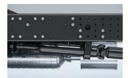
**The frame – robust and flexible.** A common hole pattern on the ladder-type frame for all models makes the Canter extremely versatile, making it easier to attach a wide range of bodies. The optional 24-volt interface and various power take-offs available ex-factory – for driving hydraulic pumps or compressor units – ensure the Canter is game for anything.
