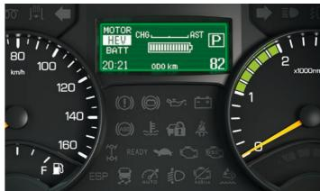
**The hybrid display.** An easily legible display keeps the driver informed of battery charge status. An indicator shows when power is being consumed or generated, providing feedback to help modify driving style for the greatest efficiency.
