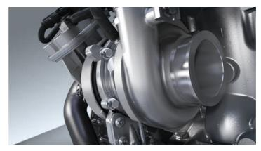
**VGT** and standard-fit exhaust brake. The variable-geometry turbocharger (VGT) optimises engine response and ensures constant high torque at low revs. The exhaust brake eases the strain on your vehicle's brake pads and discs, easing the braking system's workload on long downhill stretches.
