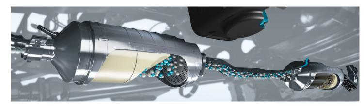
**The emissions control system.** All engine variants have a closed, maintenance-free diesel particulate filter which regenerates automatically – although you can do this manually if you need to. Exhaust gases are cleaned by a combination of oxidation catalytic converter and diesel particulate filter. Along with BlueTec® 6, the technology ensures all Canter models comply with the Euro VI standard.
