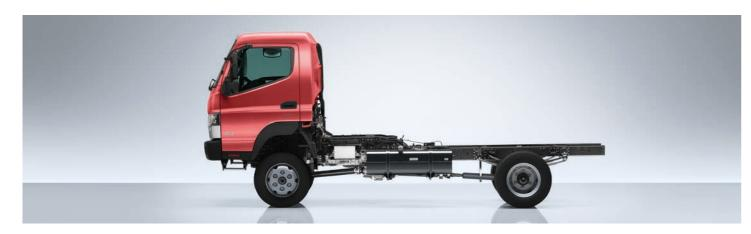
**Payload capacity.** The Canter 4×4 has a chassis load-bearing capacity of up to 3685 kg. With axle loads of up to six tonnes as well as an optional 24V interface and power take-offs ex-factory, a large choice of body options and solutions is available.
