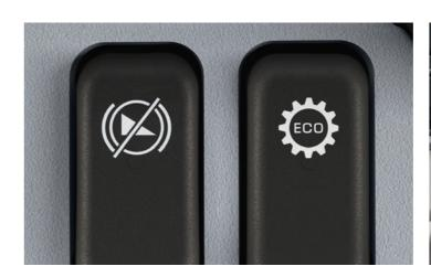
**Eco Mode and Hill Start Assist as standard.** While DUONIC® always selects the right gear for the lowest fuel consumption, Eco Mode enables further fuel savings by means of early shifting. Hill Start Assist provides support when moving off on an uphill gradient with a heavy load.
