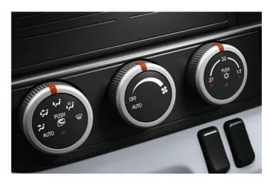
The cab's climate control. For ideal in-cab conditions we offer a choice of a manual air-conditioning system or optional automatic climate control. There's separately controlled ventilation for the crewcab.
