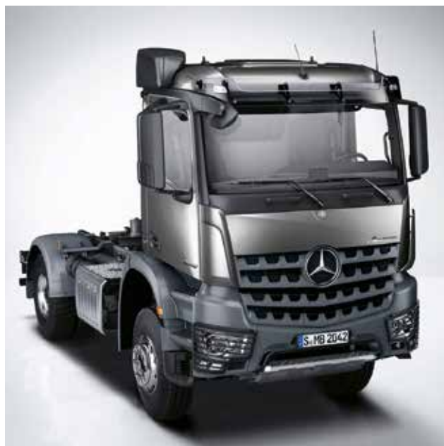
S-cab ClassicSpace 3) . The 2300 mm wide and 1700 mm long cab with an engine tunnel height of 170 mm or 320 mm is tailored to the requirements of one-man operations in construction transport and offers excellent visibility.
