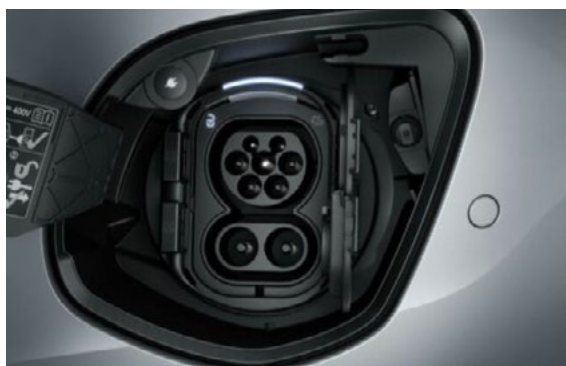
CCS rapid charging port, 80kW max. capacity.
