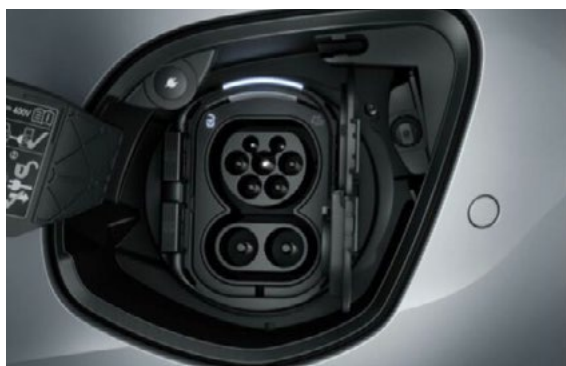
CCS rapid charging port, 80kW max. capacity.
